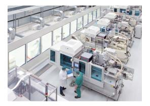
By positioning the machines outside the cleanroom, we keep the energy input per square meter of production area as low as possible.
