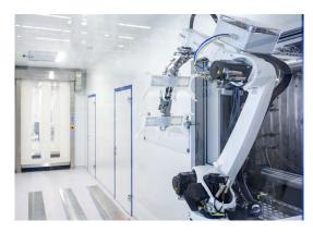
The injection-molded parts are removed from the multi-cavity mold by robots, inspected by a camera, and then stacked.
